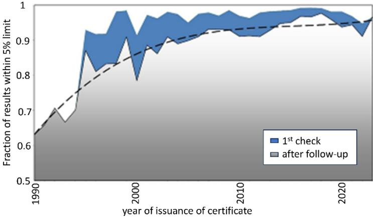
Fraction of the dosimetry audit results within the 5% acceptance limit for radiotherapy hospitals during the period 1990 – 2023. The grey area indicates the results obtained in the first check, and the blue area corresponds to the percentage of those after a subsequent follow-up.
